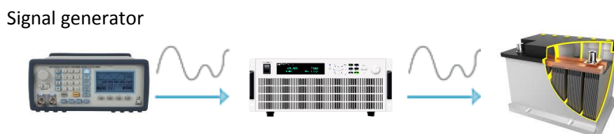
Figure 1. Load arbitrary waveforms via analog interface of IT8900A
